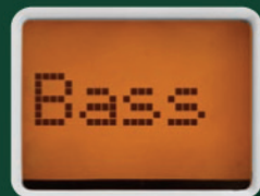
The KPL keypad uses a five-character LCD screen to display the source playing. It also allows you to adjust bass, treble, balance, loudness and volume.
